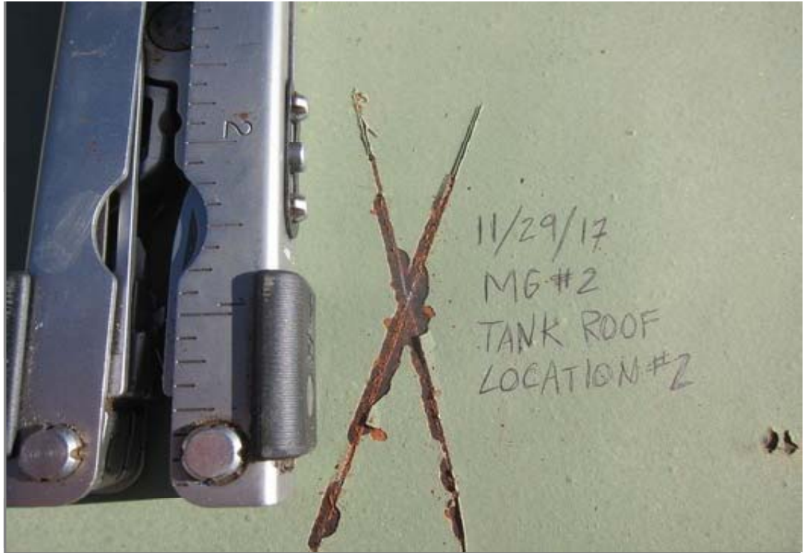
Adhesion was evaluated with a cross cut tape test and found to be 2A-3A. This location was on the exterior roof.
