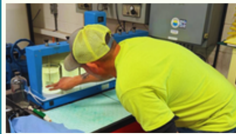
Jartests to identify or confirm correct clarifier dosing
